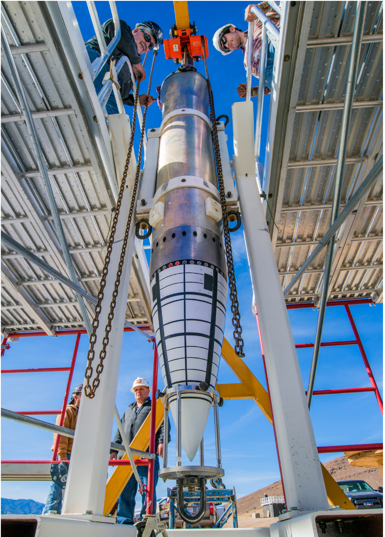
The nose assembly of a mock B61-12, mounted on an aluminum tube to replicate the body of the bomb, sits in a stand awaiting movement to Sandia National Laboratories' Davis gun, which fired the test assembly into a pool in one of a series of impact tests. Photo: US Department of Energy
