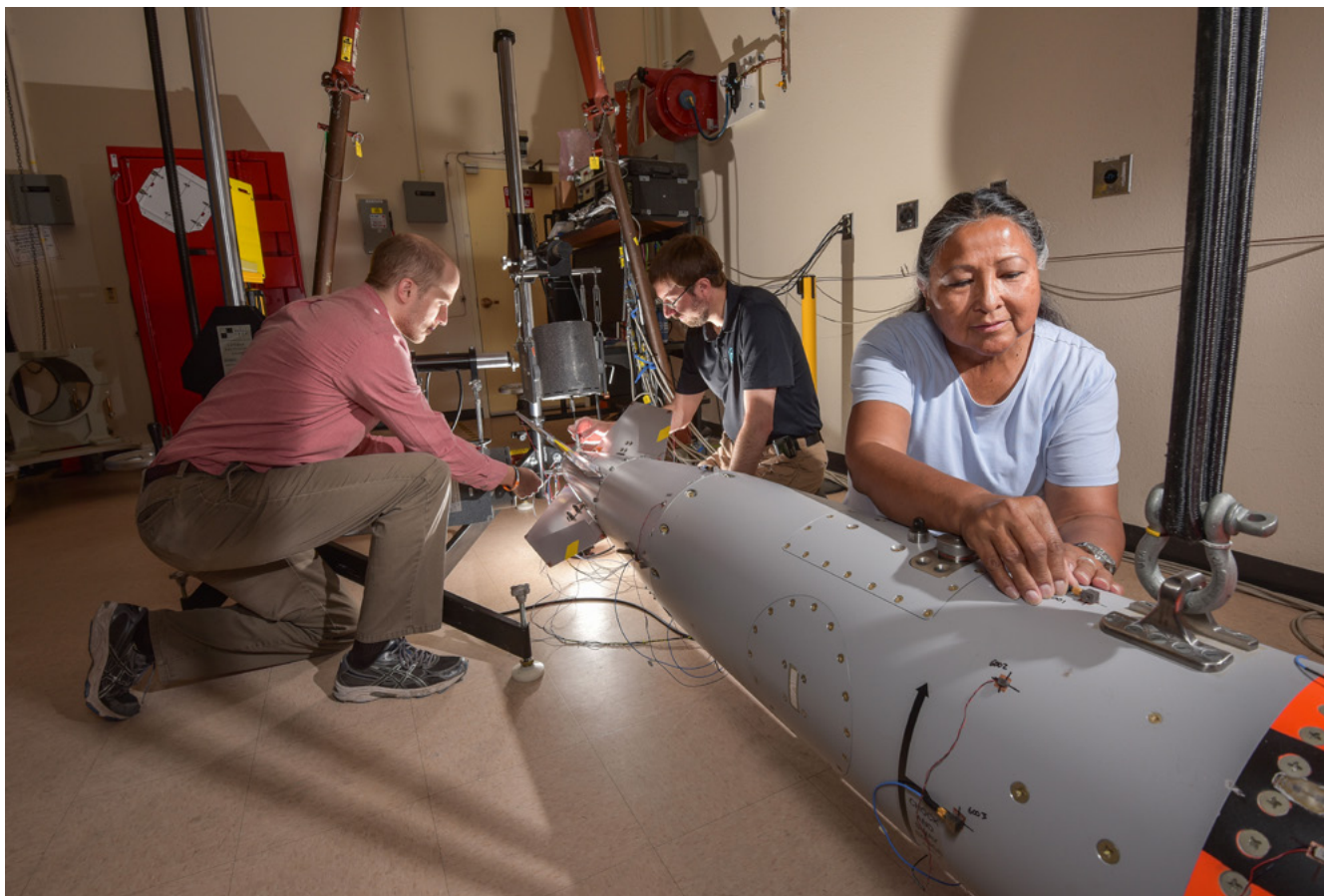
A B61-12 model goes through a vibration test to analyze structural integrity at Sandia National Laboratory. Photo: US Department of Energy
